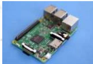
Fig -1: Raspberry Pi – Model B
