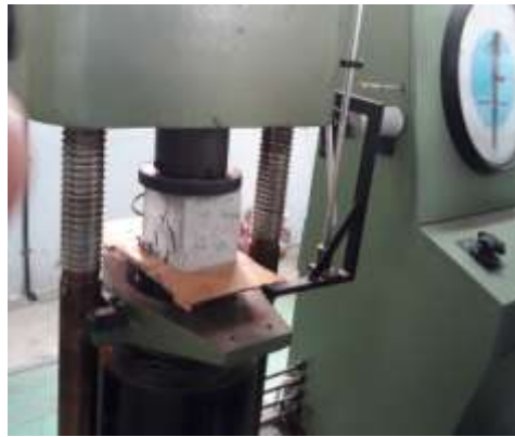
Fig 5.2 Compression strength test of concrete cube
