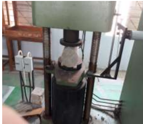
Fig 5.4 Split tensile strength test of concrete cylinder
