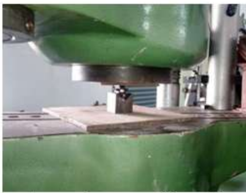
Fig.8 Experimental setup of breaking Load analysis
