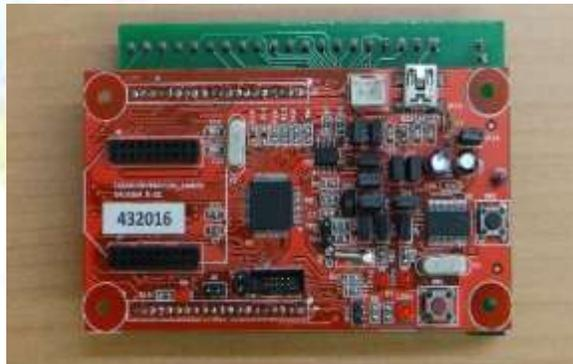
Fig.5 Fabricated VFC board connected to main board
