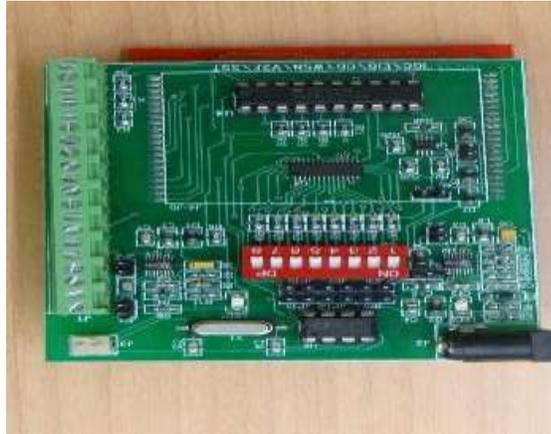
Fig. 4 Top view of fabricated VFC board
