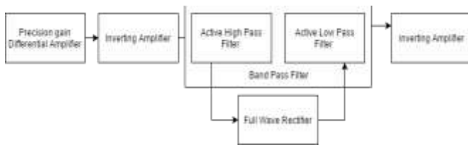
Fig. 4. Block Diagram of RMG Acquisition and Conditioning Circuit.
