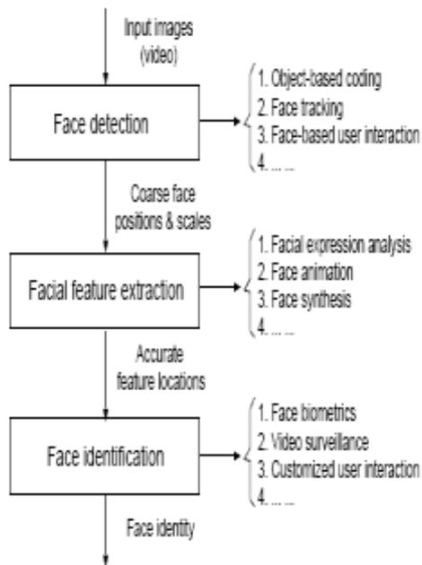
Figure 1. Framework of Face Recognition system
