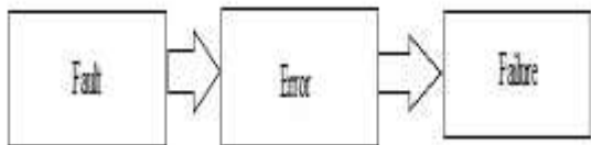
Figure 1: Consequence of a fault
