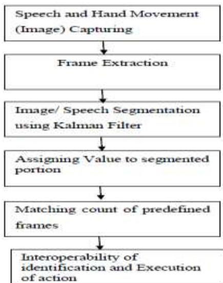
Figure 3: Design flow of intelligent adaptive interface
